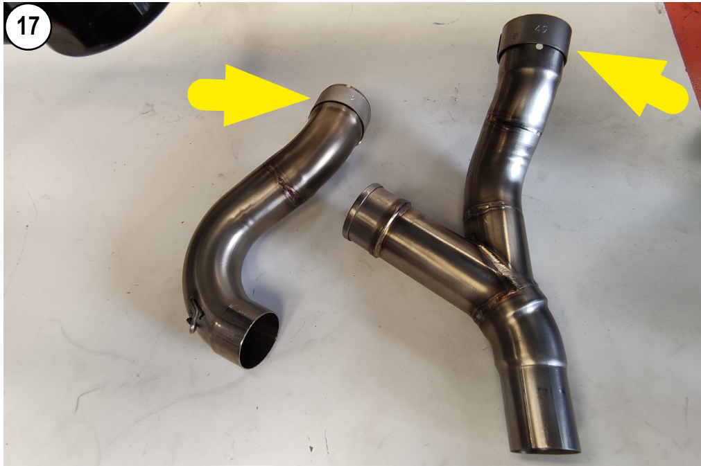
SLIP THE CLAMPS ON THE PIPES
