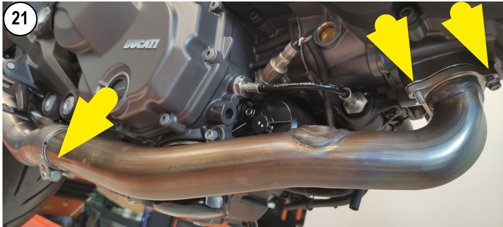
INSTALL THE FRONT PRIMARY PIPE
